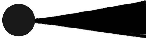
Fig. 2. Superimposed image, obtained from a video sequence, showing the extent of splitter plate motions. In this case, splitter plate length to diameter ratio, L/D = 3.0 , and Re \approx 7000 .
